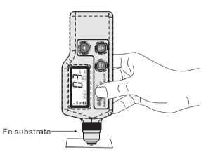
b. do not lift the detect head and press the ZERO/ON key, the buzzer will sound, that show you have complete Zero point calibrate. LCD displayed like the following picture at this time:
